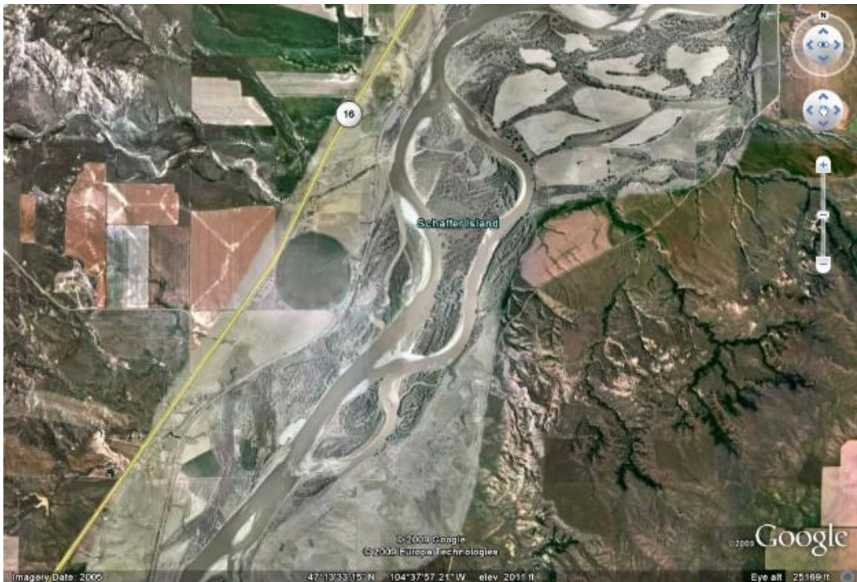
Appendix 4, Figure 1. Aerial image of the Yellowstone River upstream of the Yellowstone Diversion Intake near Schaffer Island. Note multiple channel and sandbar islands. Source: Google Earth.
